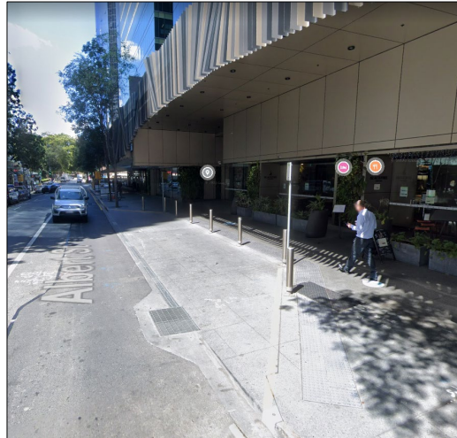
Example of integrated loading bay with flush pavement design – Capri Hotel 83 Albert Street, Brisbane
